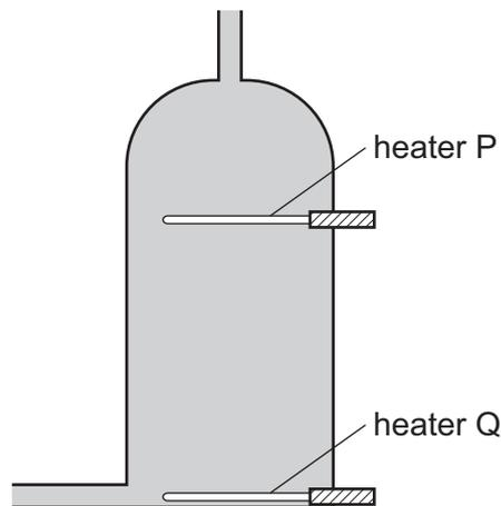
When only heater Q is switched on, it takes a long time to heat the tank of water to  $60^\circ\text{C}$ .
